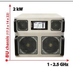
Empower RF's model 2180 is a 2000W 1GHz to 2.5GHz GaN on SiC CW amplifier with breakthrough power density. It's Multimode capabilities include AGC, ALC, MGC as well as selectable modulation modes that ease system integration. It's operating mode versatility and linear performance has the model in use for Satcom Uplink, GPS Jamming, Cyber/EW, Effects Testing, and Directed Energy research. Pulse mode with blanking is included.
