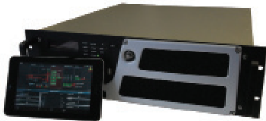
2. Using modern mobile devices, amplifier-system controls can be enhanced to increase interface functionality and control methods as these features scale in complexity. (courtesy of Res-Ingenium)
