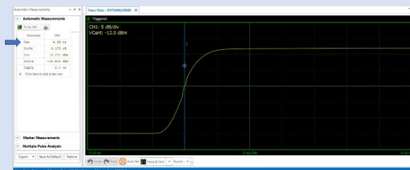
Figure S-1: Pulse rising edge with automated 10/90% rise time measurement shown by blue arrow
