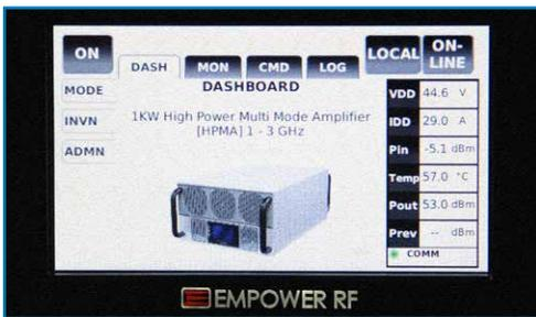
The **Dashboard** is your quick at-a-glance system status showing output power, reflected power, input power, internal temperature, transistor drain current, and transistor drain voltage.
