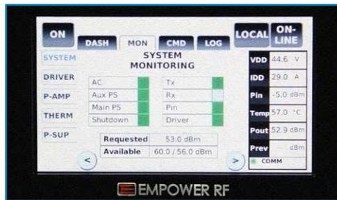
**System monitoring** shows all the at-a-glance status shown on the Dashboard and goes further with a display of major system component alarms. On any screen a swipe to the right or left takes you to the next sub tab screen.
