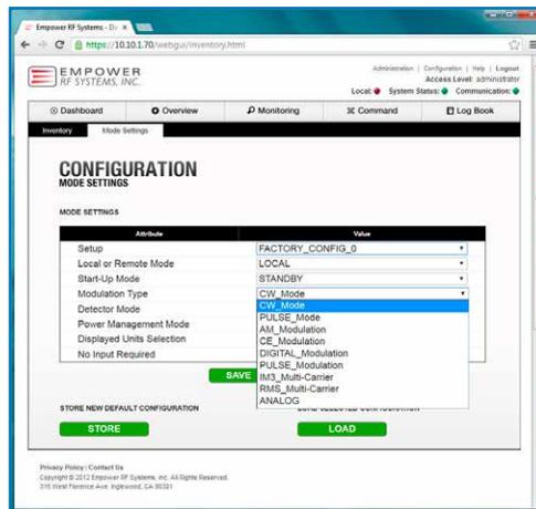
The pull down menu on the **Configuration page** makes it quick and easy to set the proper input modulation scheme to ensure both the input power and output power metering is accurate and not "for indication purposes only".
