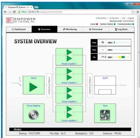
Here is the **GUI Overview page** seen through the web browser of a peer connected PC or via Lan. Its more than just a block diagram graphic since each block is click-able to drill down to system health parameters.
