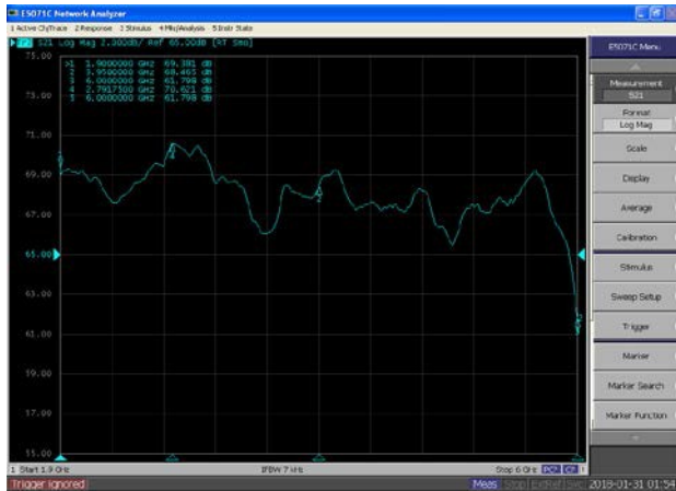
Plot 3 – Gain Adjustment Range @ P_{IN} = -30\text{dBm}
