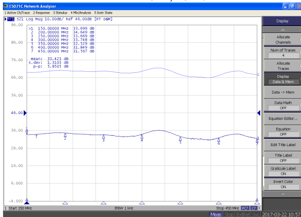
Plot 3 – Gain Adjustment Range @ P_{IN} = -30\text{dBm} Top Curve: Maximum Gain Bottom Curve: Minimum Gain Reference: 46dB, 10dB/div.
