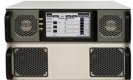
With a proprietary scalable architecture this amplifier can be easily upgraded to our 4KW 2207 or 8KW 2208 by adding either two or four additional 3U power blocks and one combiner providing you with a cost effective upgrade path. For those who own two 2206's, only one additional combiner is needed to configure a 4KW system.
