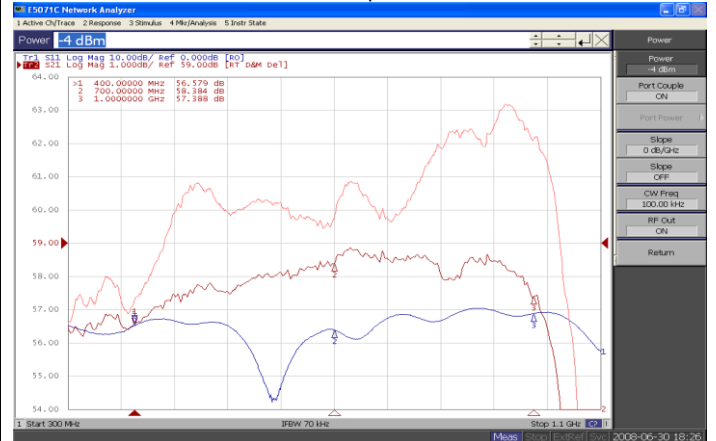
Plot 2 - Gain @ Psat with 1097 Driver Top Curve: Power Gain @ Pin = -20.0dBm Middle curve: Power Gain @ Psat, Pin = -4.0dBm Reference: 59dB, 1dB/Div Bottom Curve: Input Return Loss
