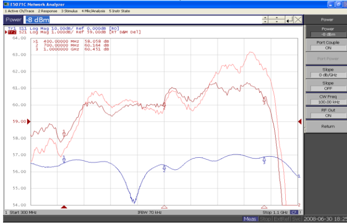
Plot 1 - Gain @ P1dB with 1097 Driver Top Curve: Power Gain @ Pin = -20dBm Middle curve: Power Gain @ P1dB, Pin = -7.0dBm Reference: 59dB, 1dB/Div Bottom Curve: Input Return Loss
