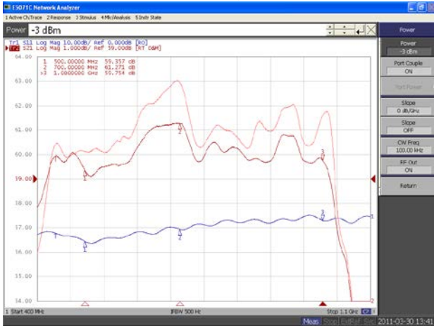
Plot 3 – Gain Adjustment Range Top Curve: Maximum Gain @ P IN = -20dBm Middle Curve: Minimum Gain @ P IN = -20dBm Reference: 30dB, 10dB/div. Bottom Curve: Input Return Loss @ Minimum Gain Reference: 0dB, 10dB/div.
