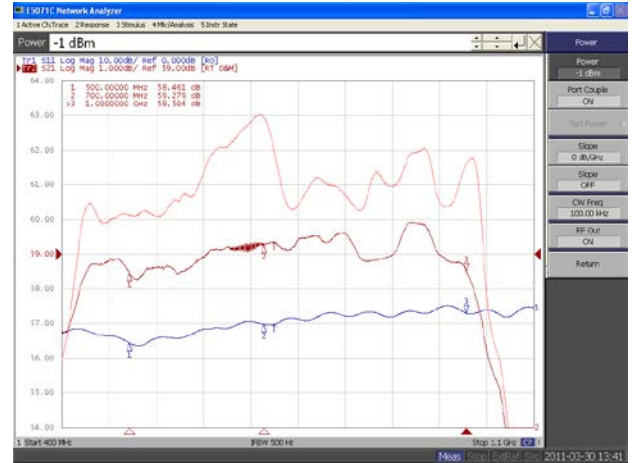
Plot 4 – Mode ALC @ 250W and 50W Top Curve: ALC @ 250W P IN = 0dBm Bottom Curve: ALC @ 50W P IN = 0dBm Reference: 50.5dB, 1dB/Div. Middle Curve: Input Return Loss Reference: 0dB, 10dB/Div.
