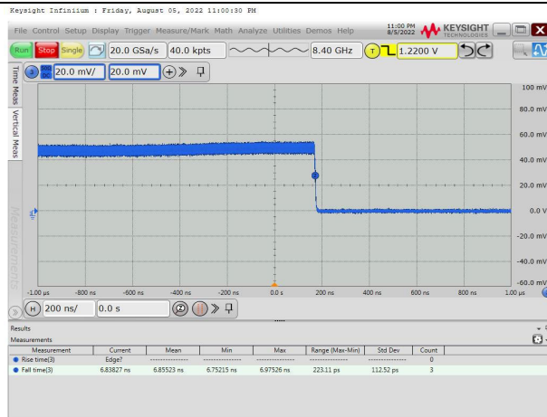
Plot 15 - Pulse Performance - Typical Fall time- 2µs PW and DC=1%
