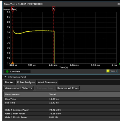
Plot 11 - Pulse Performance - Typical Fall time-2ms PW and DC=10%
