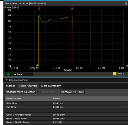
Plot 15 - Pulse Performance - Typical Fall time- 2µs PW and DC=1%
