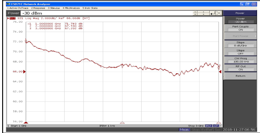
Plot 3 - Input Return Loss Top Curve: Power Gain @ Constant P_{IN} = -30\text{dBm} Reference: 0dB, 10dB/Div.
