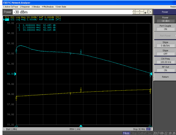
Plot 3 – Gain Adjustment Range @ P_{IN} = -30\text{dBm}
